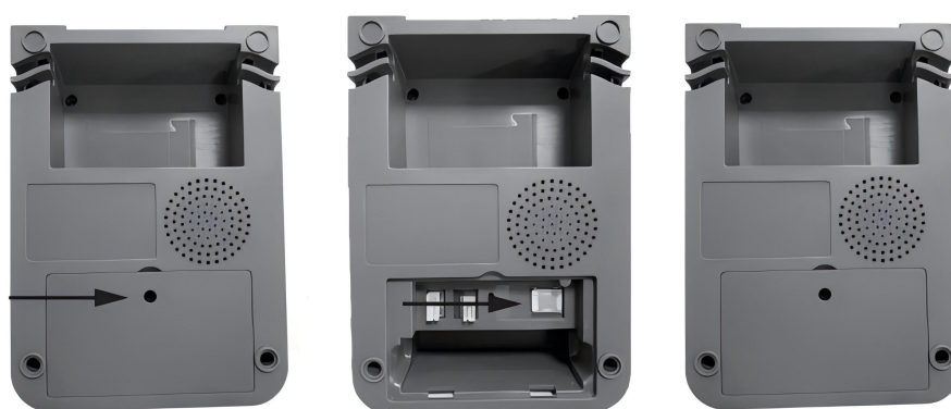
Cover removal, SIM insertion and cover replacement, from top to bottom.
